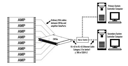
To create the more complex distributed star topologies needed for larger systems, use additional hubs or switches. Some have special uplink ports for connecting to other hubs or switches via a standard Ethernet cable. If the hubs or switches do not have uplink ports, then the hub-to-hub or switch-toswitch connection should use a crossovertype Ethernet cable.
